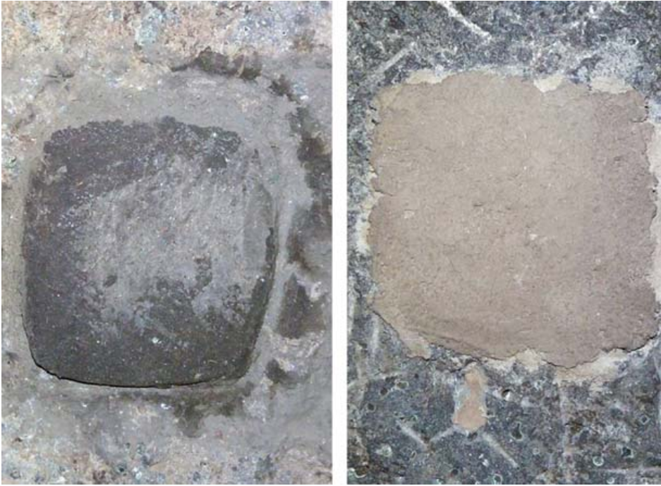
Fig. 4. Application of mud mortar on basaltic stone
