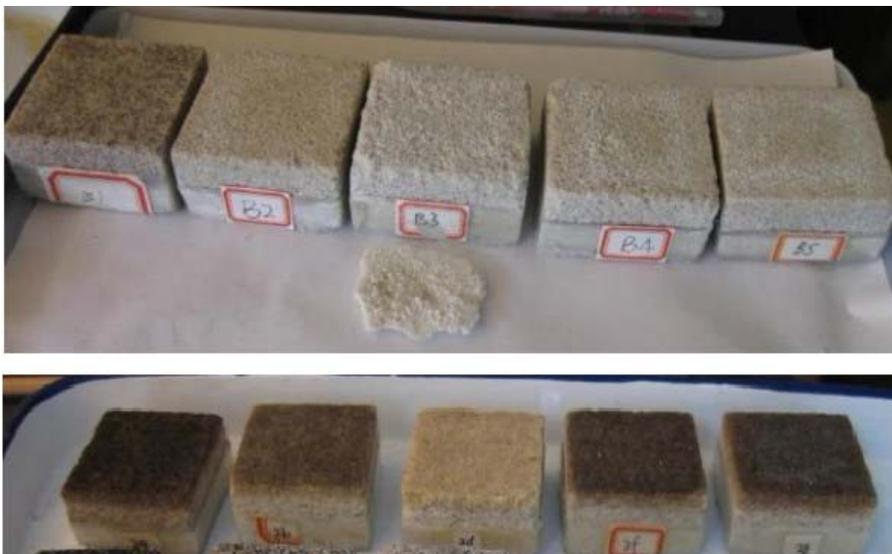
**Fig. 10.** Picture of sandstone samples after salt destruction cycle
