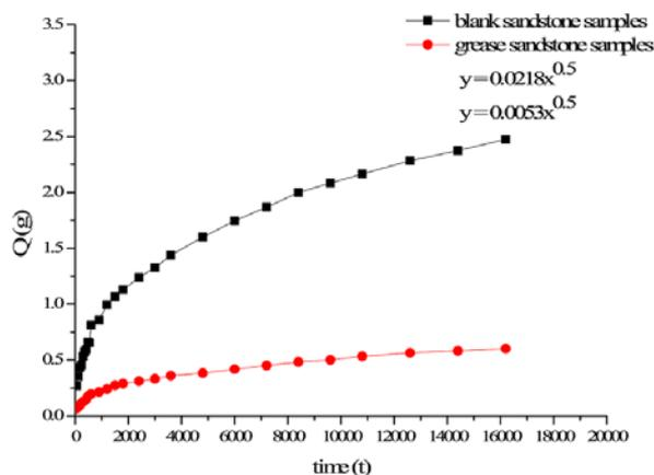
Fig. 11. Amount of water absorbed (g) by capillarity as a function of time (s) in blank and grease sandstone samples
