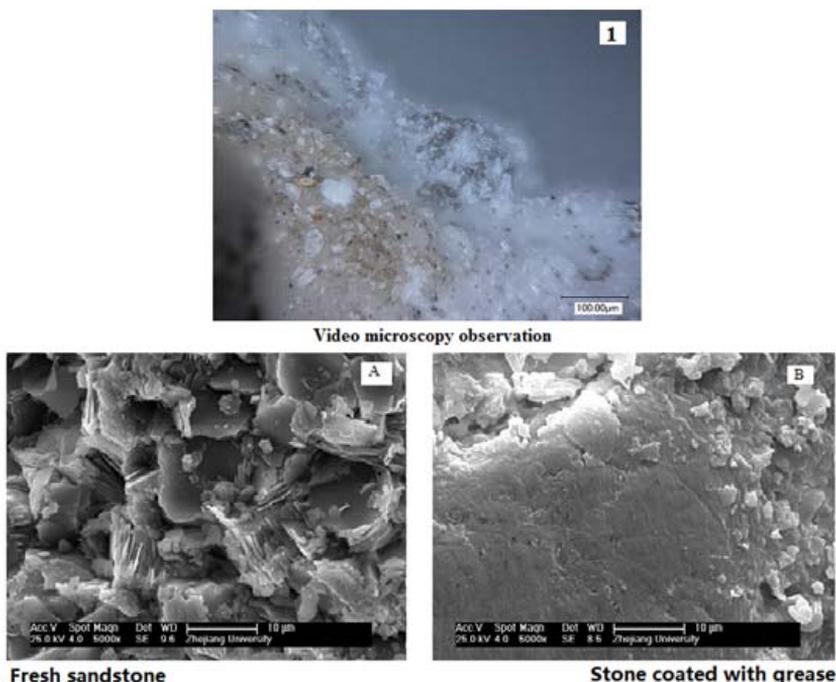
**Fig. 5.** Microscopic observation and analysis of real sandstone samples from Yungang Grottoes
