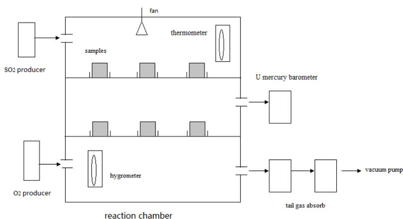
Fig. 4. Diagram representing SO<sub>2</sub> corrosion test chamber
