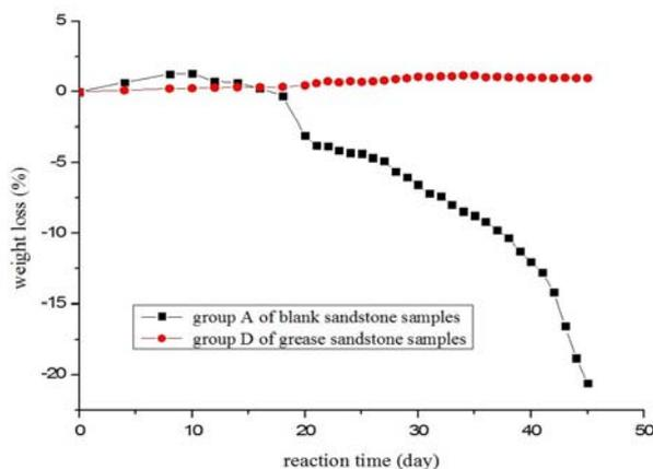
**Fig. 8.** Weight loss versus reaction time for blank and grease sandstone samples in the SO<sub>2</sub> corrosion test.
