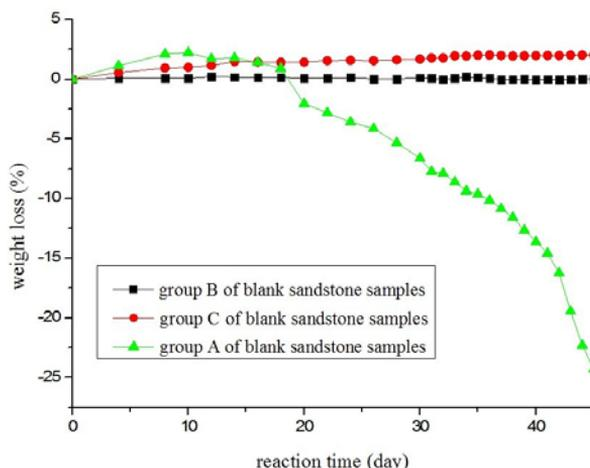
**Fig. 7.** Weight loss versus reaction time for three groups of blank sandstone samples in the SO<sub>2</sub> corrosion test.
