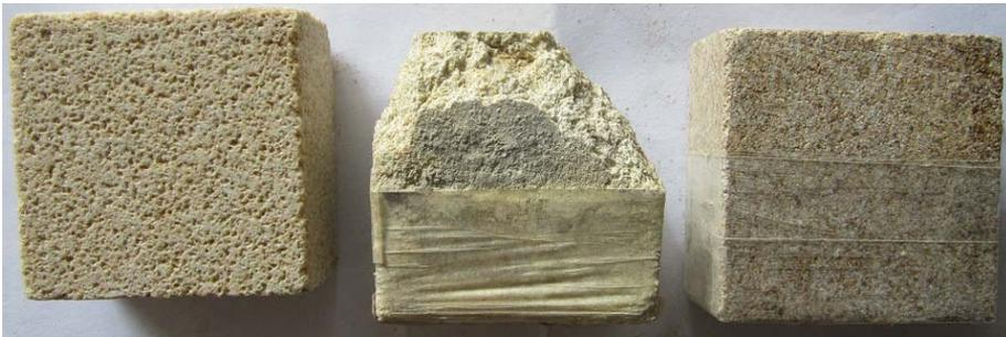
**Fig. 9.** (Left) fresh sandstone; (Middle) blank sandstone sample taking part in wetting, SO<sub>2</sub> corrosion and drying tests; (Right) grease sandstone sample taking part in wetting, SO<sub>2</sub> corrosion and drying tests
