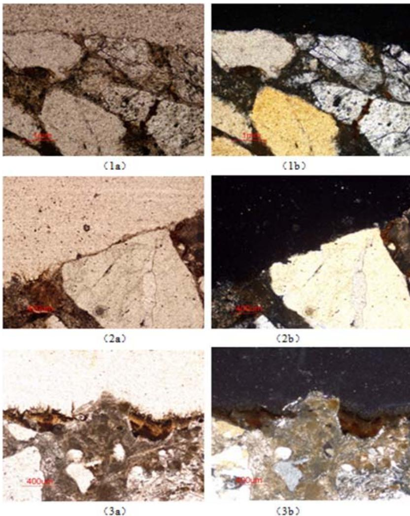
Fig. 6. Polarized cross-section images of the grease stains
