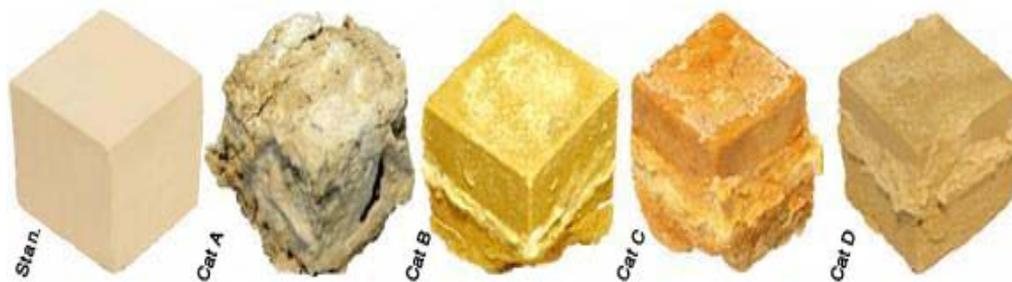
Fig. 2. The visual appearances of affected samples compared with standard sample
