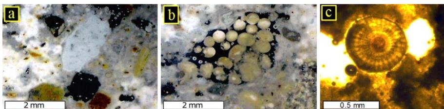
**Fig. 22.** Thin section of the external wall plaster showing a rich background of calcite, gypsum clusters, stone fragments and spherical objects (fossils) (OM image) (a and b). Spherical objects (fossils) in calcite background (CN) (c).
