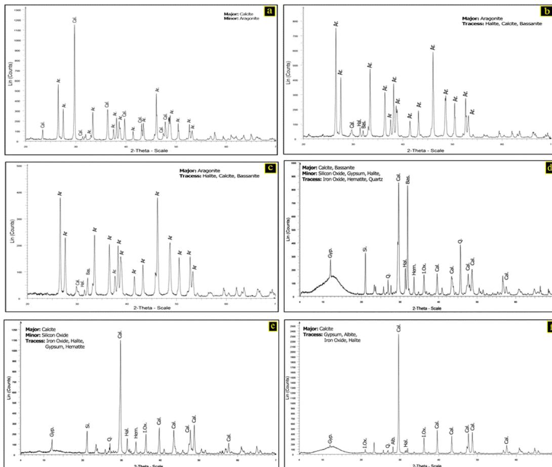
**Fig. 29.** X-ray patterns of the identified minerals in the studied building materials samples: (a) - Honeycomb coral limestone sample, (b) - Great star coral limestone sample, (c) - Brain coral limestone sample, (d) - Mortar sample, (e) - External wall plaster sample and (f) - Internal wall plaster sample.
