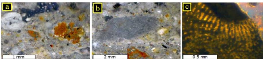
Fig. 20. Thin section of the mortar showing a rich background of calcite, gypsum clusters and stones fragments (OM image) (a and b), coral limestone fragment, aragonite (C.N.) (c)
