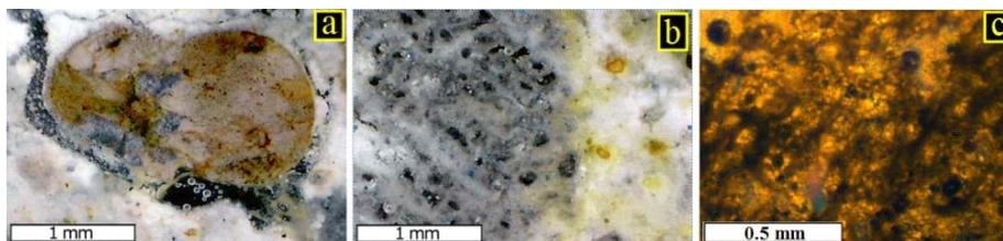
**Fig. 24.** (a and b) Thin section of the internal wall plaster showing calcite background, quartz grains, coral stone fragments (OM image), (c) Calcite and gypsum matrix, (CN)
