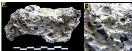
**Fig. 23.** (a and b) Qasr El-Emara internal wall plaster containing black stone fragments.
