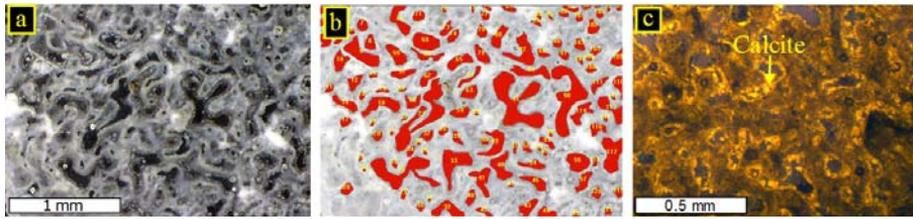
Fig. 14. Cross section of fine texture honeycomb coral limestone showing stone porosity (OM image) (a and b), The arrows indicate calcite rims and the darker color of the coralline aragonite (CN) (c)
