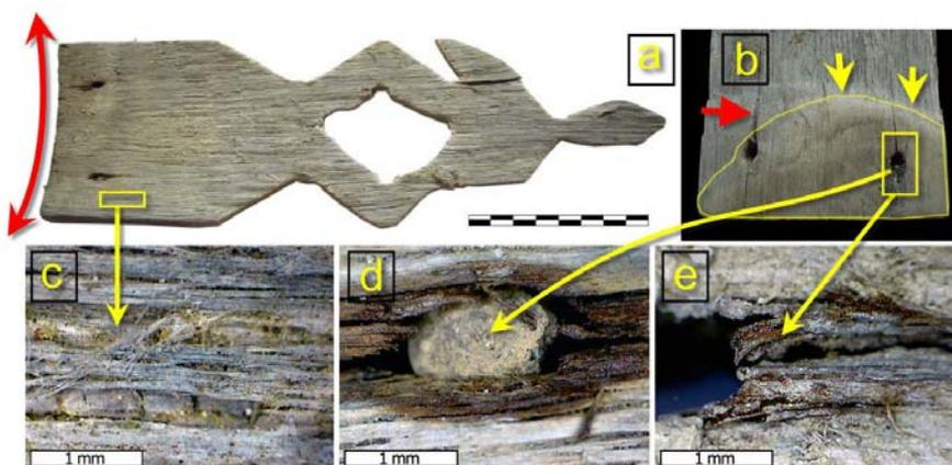
**Fig. 27.** Outer surface of oriel decorated wooden element, which was affected by warping, cracks and superficial damage (a); the internal surface has rust stains, due to use of iron nails (b); enlarged image of cracks (c); enlarged image of rust stains (d and e).
