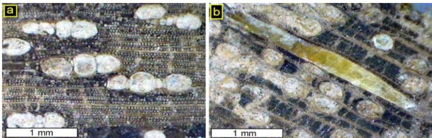
**Fig. 28.** Cross section of the timber sample which shows vessels (perforation plate) (a); longitudinal tangential section, which shows longitudinal tracheas filling with resin used to plug up the wood pores (b).
