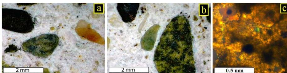
**Fig. 25.** (a and b) Thin section of the internal wall plaster showing calcite background, quartz grains, stone fragments in different shapes and colors (OM image) (c) calcite and gypsum matrix, (CN)
