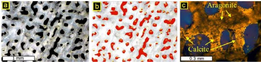
Fig. 13. Cross section of fine texture honeycomb coral limestone showing stone porosity (OM image) (a and b), The arrows indicate calcite rims and the darker color of the coralline aragonite (CN) (c)
