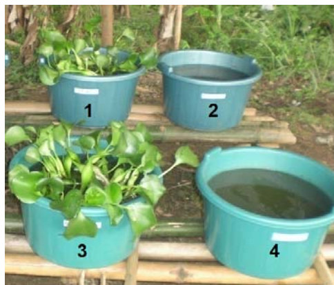
Fig. 2. Experimental device located at the University of Abobo-Adjamé: (1) and (4) Eichhornia crassipes in industrial wastewater effluents, (2) and (3) Same industrial wastewater effluents without any plants.
