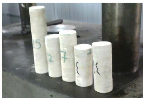
Fig. 5. Some Core Samples after Preparation for Mechanical Testing
