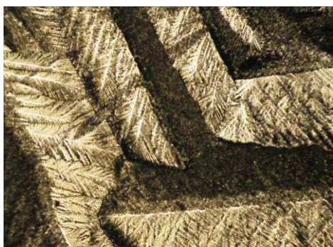
Fig. 7. The surface morphology obtained in baths of Zn + 0,36% Bi, 50X
