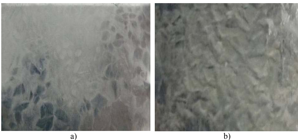
Fig. 3 The macrostructure of the galvanized surfaces, 50X [3]: a) smooth aspect, b) coarse aspect
