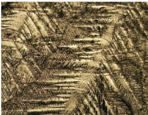
Fig. 6. The surface morphology obtained in hot-dips Zn + 0,27% Bi, 50X
