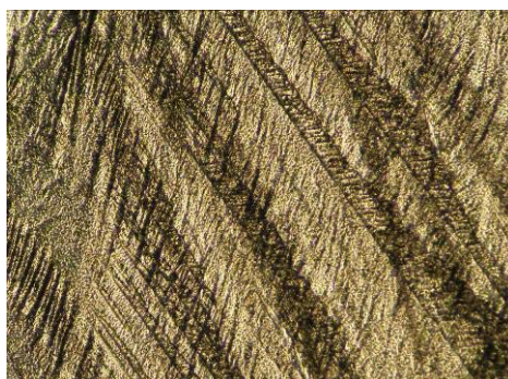
Fig. 8. The surface morphology obtained in baths of Zn + 0,52% Bi, 50X
