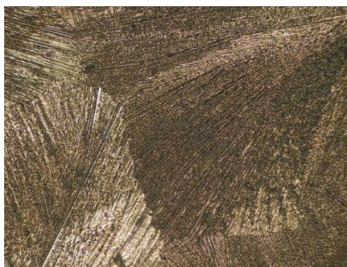
Fig. 4. The coating morphology with Zn-Ni-Pb-Sn, 50X
