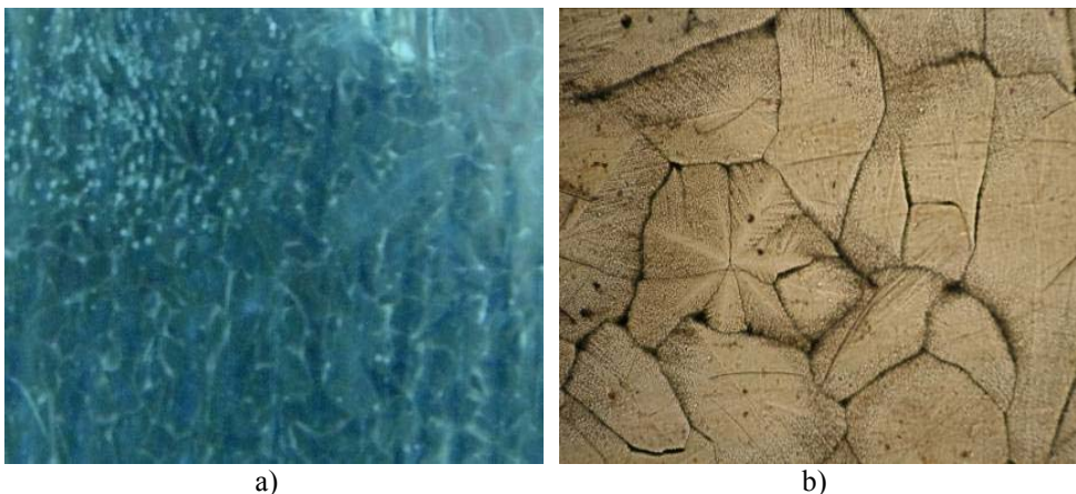
Fig. 2 The surface morphology of the straps coated with zinc without „zinc flowers” [3]: a) macroscopic 5X; b) microscopic, 50X
