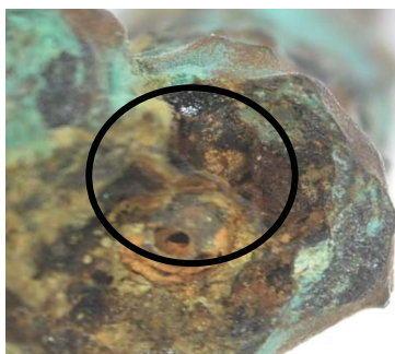
Fig. 27. Iron pin in the form of a tube empty on the inside, 40X.
