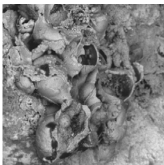
Fig. 15. Vesicant-type formations, 500X.
