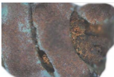
Fig. 25. Copper alloys coils wound up on the iron pin, 40X.
