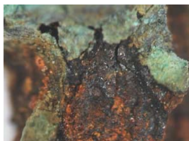
Fig. 11. Exfoliated foils from the corrosion crust, 40X.
