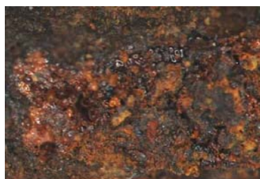
Fig. 7. Secondary and tertiary chemical compounds in the corrosion crust, 60X.
