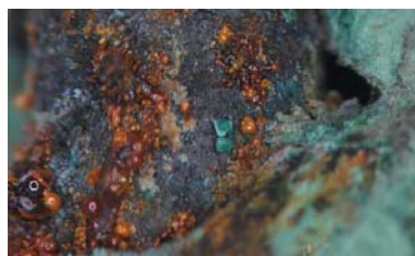
Fig 9. Vesicant-type formations, 60X.
