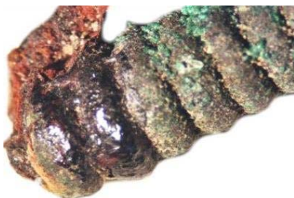
Fig. 34. Corrosion crust on the spring, inventory number 12836.
