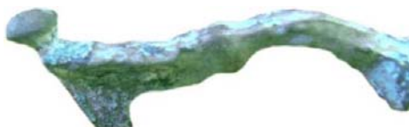
Fig. 23. External corrosion layer on the fibula body.
