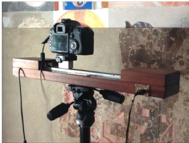
Fig. 4. Micro-photogrammetry system (by Menci Software Srl, Arezzo, Italy).
