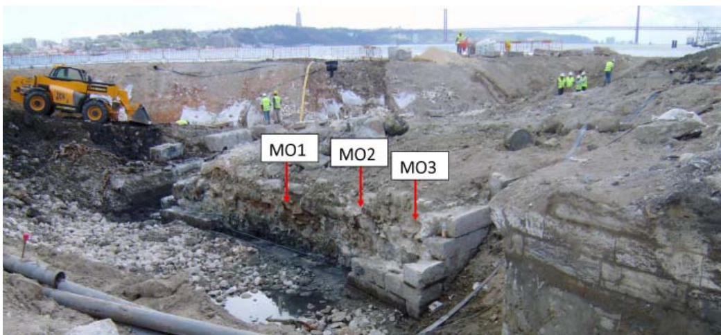
Fig. 3. Sampling of mortars at the core of Cais das Colunas . West elevation, 2008.
