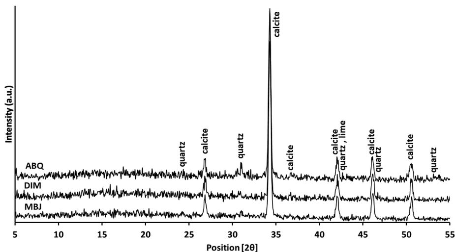
Fig. 4. X-ray diffraction patterns for the indicated bulk mortar samples
