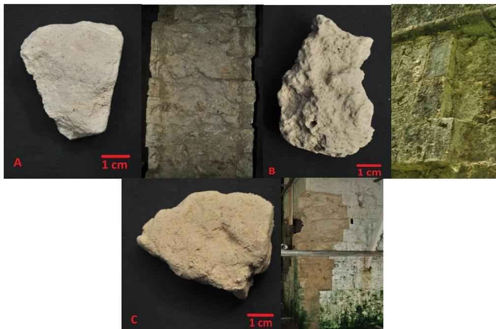
**Fig. 2.** The rubble mortar samples used in this study from (A) Alburquerque church convent, (B) Dimiao mortuary chapel, and (C) Maribojoc church convent
