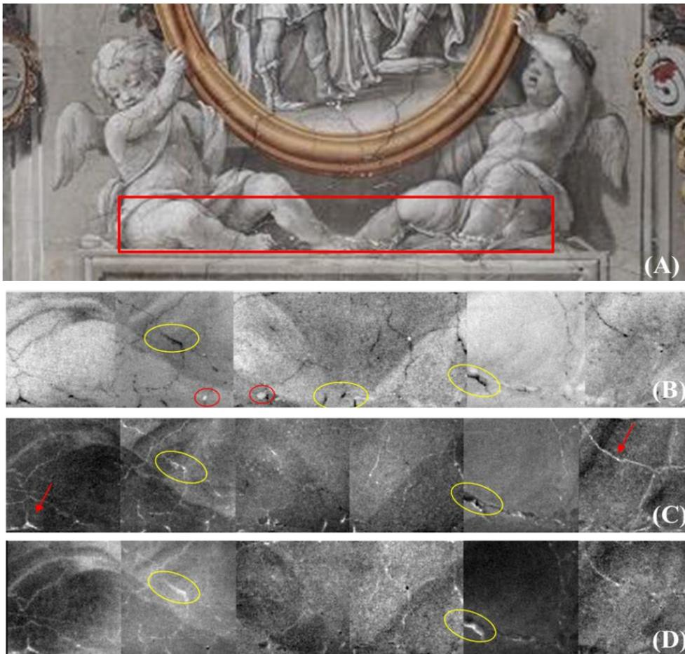
**Fig. 5.** Results of PuCT analysis before restoration. (A) The investigated area in the red frame; (B) thermogram at time 1.5s; (C) thermogram at time 3.5s; and (D) thermogram at time 12.5s
