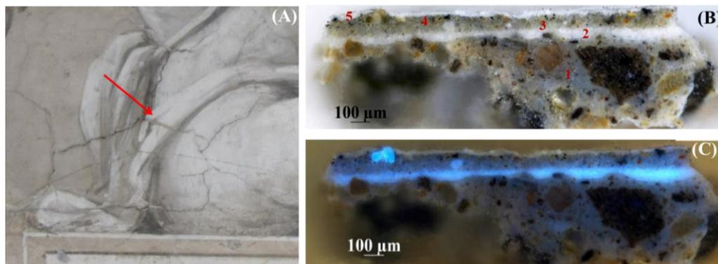
**Fig. 6.** Microstratigraphic analysis: (A) image of the sampling point; (B) cross-section under reflected light; and (C) the same cross-section under UV fluorescence
