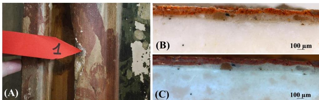
**Fig. 7.** Microstratigraphic analysis on the false marble decoration in the stucco arch: (A) image of the sampling point; (B) cross-section under reflected light; (C) the same cross-section under UV fluorescence
