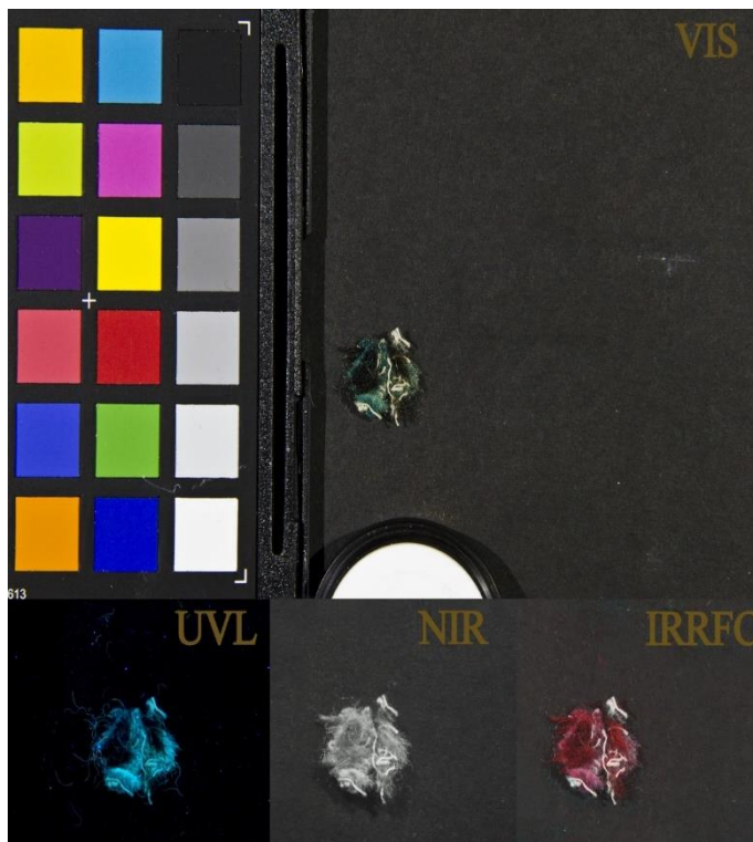
Fig. 8. Visible reflected (VIS); ultraviolet induced visible luminescence (UVL); near-infrared reflected (NIR) Infrared reflected false colour (IRRFC) images of the textile fragment (C) of an Islamic carpet, Cairo Egyptian Museum
