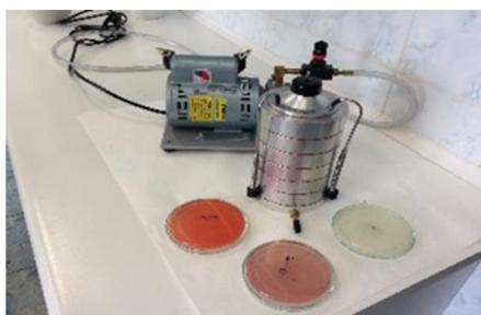
Fig. 4. The cascade impactor and Petri dishes
