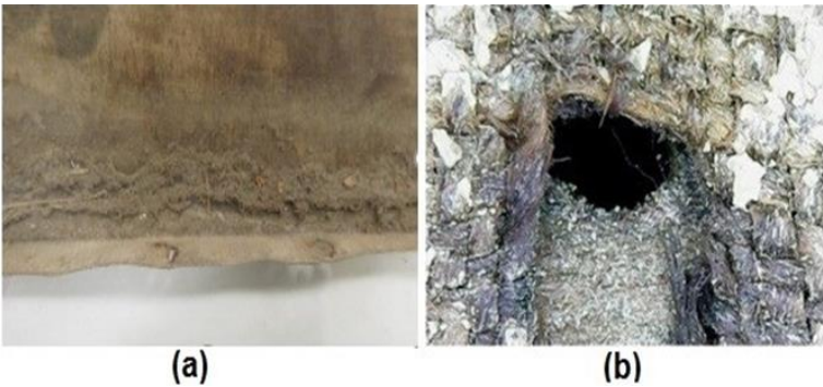
Fig. 14. Manifestations of support layer deterioration: (a) Dirt; (b) Holes
