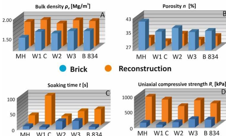
**Fig. 10.** Comparison of physical and mechanical properties of mud bricks and reconstructed brick material (see text for details): A – bulk density, B – porosity, C – soaking, D – uniaxial compressive strength. Symbols of objects as in Figure 2B.
