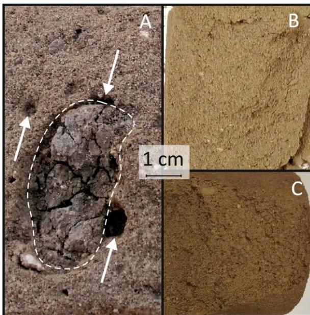
**Fig. 9.** Brick material structure from Building 834 in macro scale (see text for details): A – heterogeneous structure of mud brick, note large clay clast with desiccation cracks (surrounded by dashed line) and large pores (arrowed), B and C – reconstructed homogeneous structure of mud brick material.
