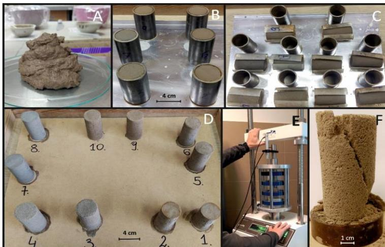
**Fig. 5.** Methodology of reconstructed brick material analysis: A – preparation of mixture, B – material placed in steel pipes, C – drying of formed samples, D – preparation of samples for compressive strength analysis, E – uniaxial compressive strength analysis, F – sample destruction after compressive strength analysis.
