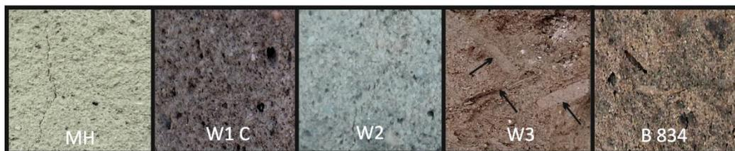
**Fig. 7.** Mud brick colours: MH – light grey, W1 C – grey-brown, W2 – light grey, W3 – brown (arrows indicate imprints of plant fragments), B 834 – dark brown. Symbols of objects as in Fig. 2B.
