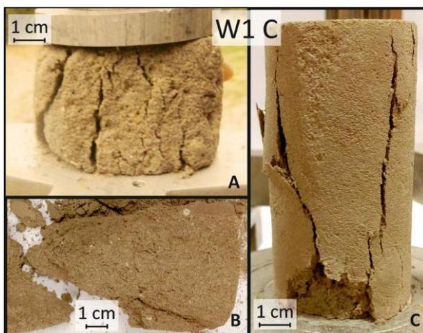
**Fig. 11.** Type of sample destruction after uniaxial compression test of W1 C (see text for details): A – mud brick, B and C – reconstructed mud brick material. Symbol of object as in Figure 2B.
