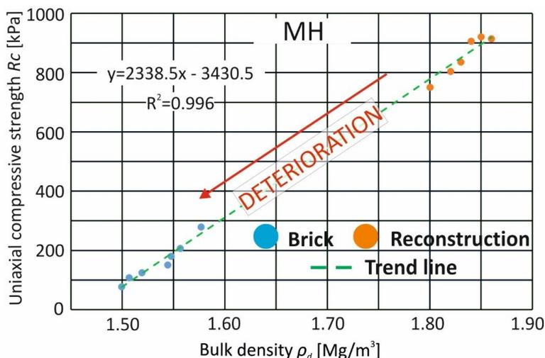
Fig. 12. Influence of deterioration processes on the mud bricks properties from Mustafa's House (MH). Correlation of uniaxial compressive strength with bulk density (see text for details).
