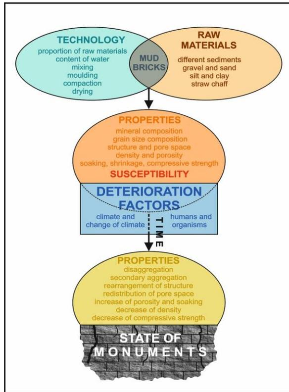
Fig. 13. Diagram showing the influence of deterioration processes on the preservation of mud brick architecture.
