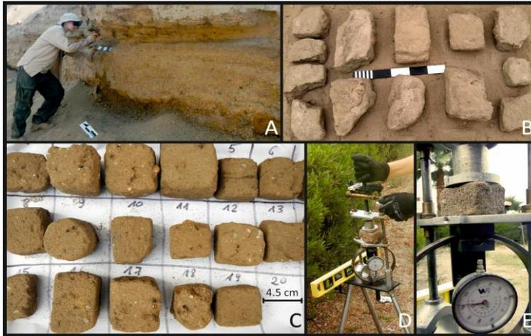
**Fig. 4.** Methodology of mud bricks analysis: A – fragment of “Wall 1”, B – selected bricks, C – samples for laboratory analysis, D – general view of apparatus for compressive strength analysis, E – sample during analysis of uniaxial compressive strength.
