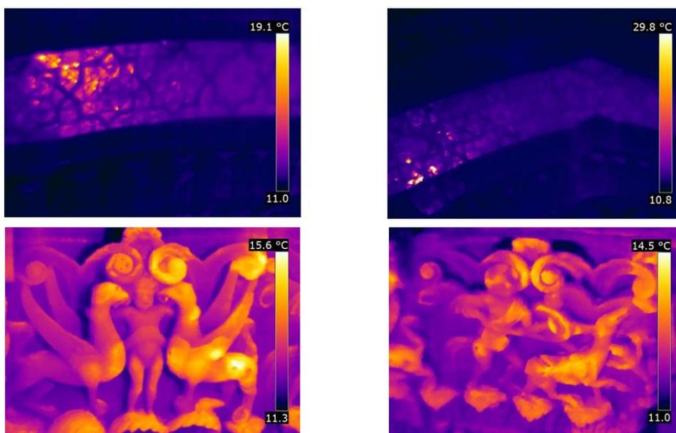
**Fig. 4.** IR Thermography: mapping of thermal anomalies (detachments, cracks, integrations) on mosaic decoration and carved marble to provide a support for securing and consolidating the precious surfaces.
