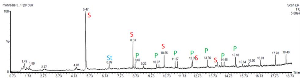
**Fig. 6.** Py-GC/MS analysis: S: Polydimethylsiloxane (PDMS); P: Aliphatic hydrocarbons; St: Styrene
