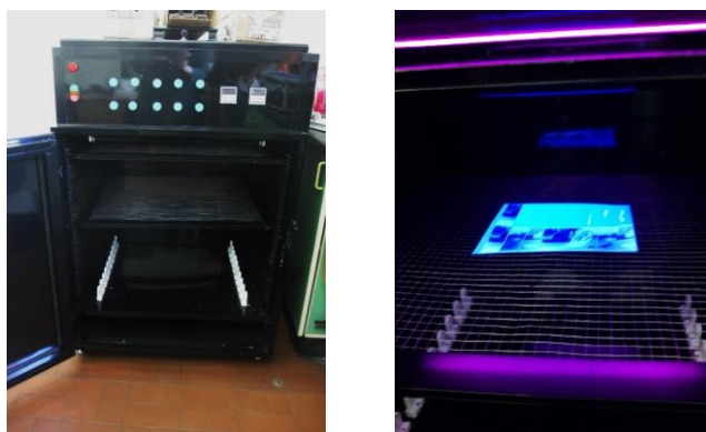
Fig. 2. Shows UV exposure device while placing samples inside with constant distance between the lamp and the photograph
