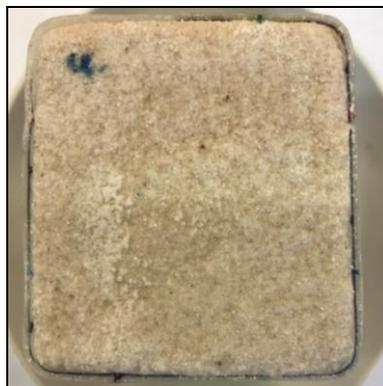
**Fig. 14.** Salt crust and efflorescence formed at the end of drying process on sample 11-7 salinated with salt mixture and treated with 0% inhibitor solution
