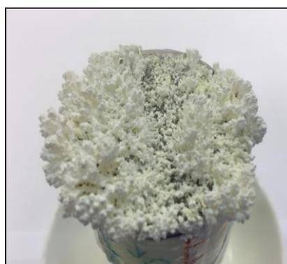
**Fig. 7.** Efflorescences formed at the end of drying process on sample 7-5 salinated with saturated solution of NaCl and treated with 1% inhibitor solution
