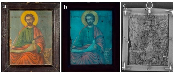
Fig. 4. the difference images of the wood painted showing the large insect tunnels and holes in wooden panel of icon: a) visible; b) UV luminescence; c) Radiographic image
