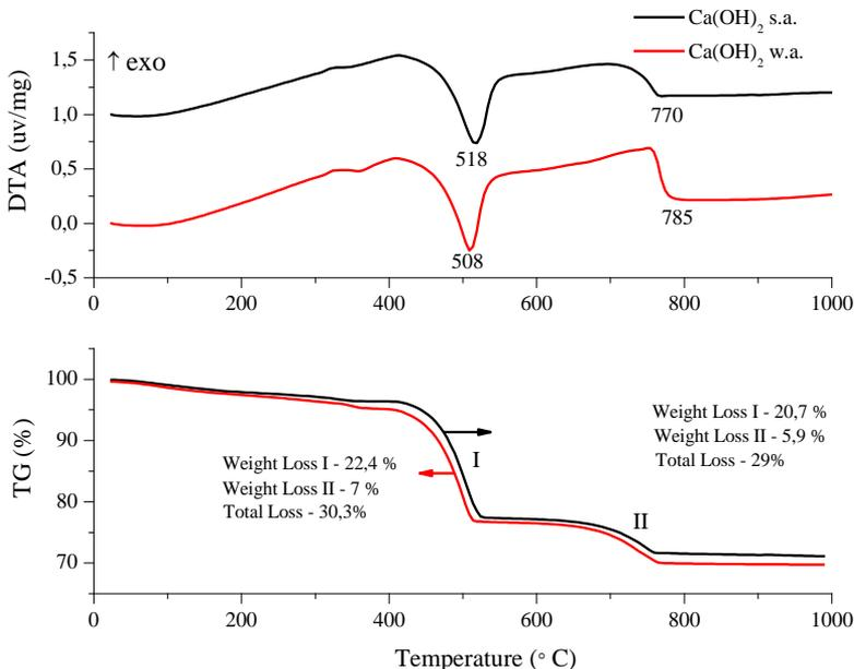
Fig. 3 DTA / TG curves of Ca(OH)<sub>2</sub> obtained by precipitation from strong acid medium (Ca (OH)<sub>2</sub> s.a.) and weak acid medium (Ca(OH)<sub>2</sub> w.a.)
