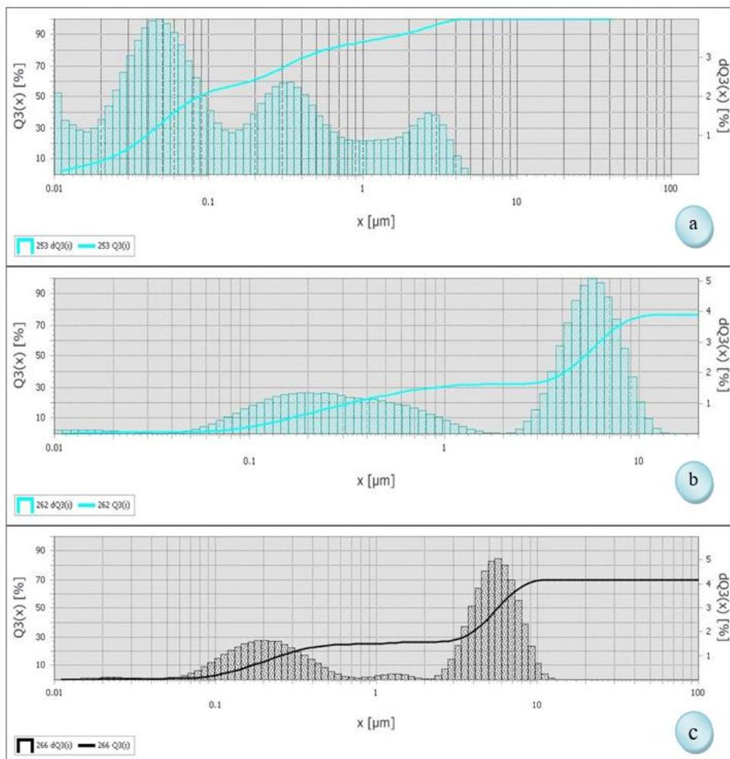
**Fig. 1** Particle-size distribution of nano- $\text{Ca}(\text{OH})_2$  synthesised from strong acid media (a), weak acid media (b) and commercial hydrated lime (c)
