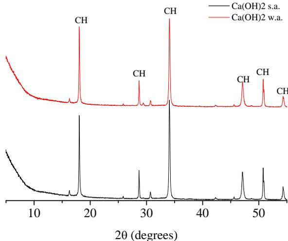
Fig. 2 XRD patterns of Ca(OH)<sub>2</sub> obtained from both strong and weak acidified solutions
