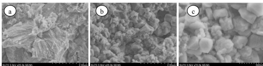
**Fig. 4** SEM images of CHL (a) and  $\text{Ca}(\text{OH})_2$  obtained by eggshells valorisation from strong acidified solution (b and c)
