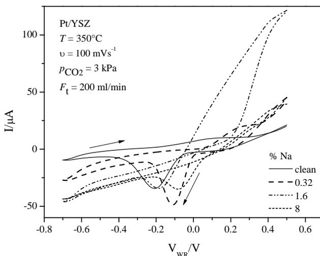
Fig. 4. Pt cyclic voltammogram of Na-modified Pt/YSZ at different Na coverage
