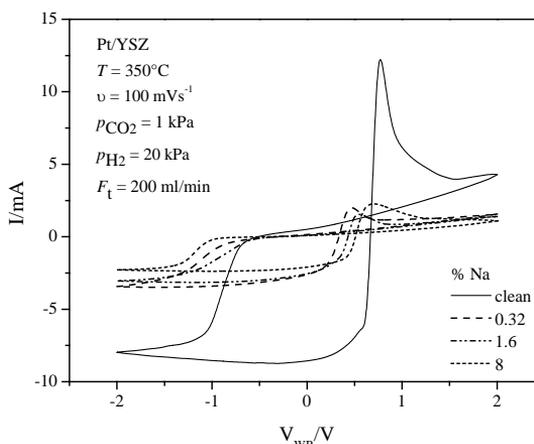
Fig. 6. Effect of sodium loadings on cyclic voltammogram of Pt under reactive conditions
