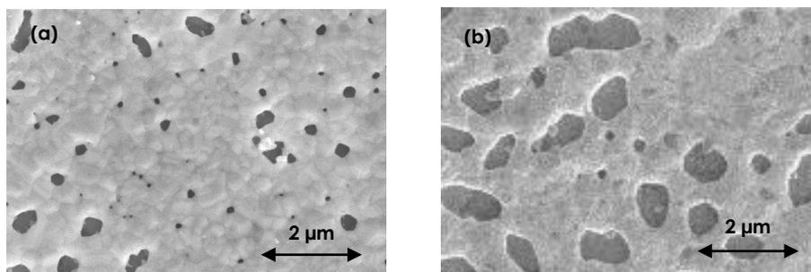
**Fig. 1.** FESEM images of (a) fresh and (b) used Pt/YSZ at 10,000 $\times$  magnifications
