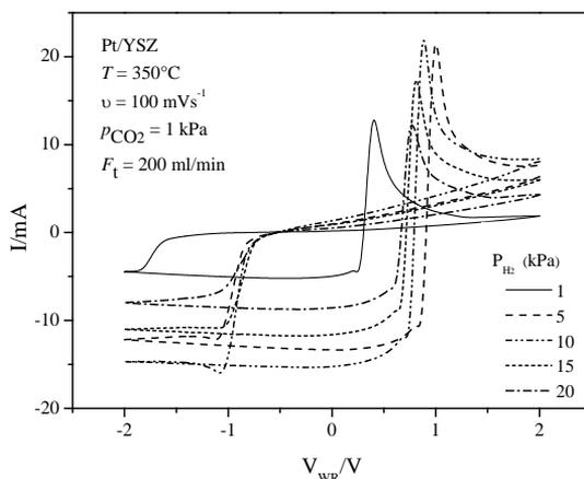
Fig. 5. Effect of varied  $H_2$  partial pressure on cyclic voltammogram of 'clean' Pt films under reactive conditions
