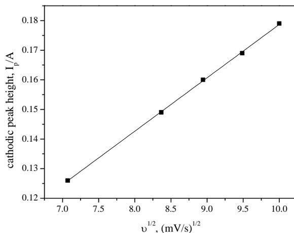
**Fig. 3.** Relationship between cathodic peak height,  $I_{pc}/A$ , and square root of the scan rate,  $v^{1/2}$
