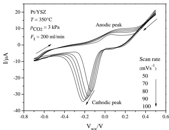
**Fig. 2.** The features of Pt cyclic voltammogram of 'clean' Pt films deposited on YSZ pellet at difference scan rates
