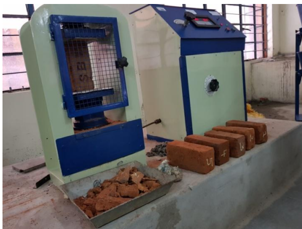
Fig. 7. Compression Testing of Modern Bricks
