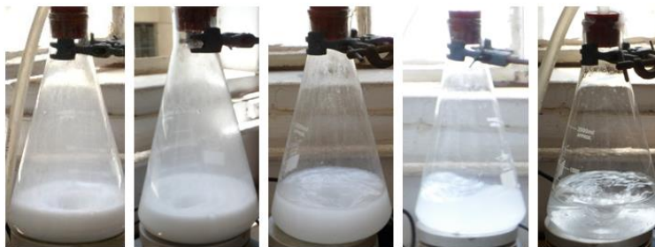
Fig.1. Stages of the preparation of aqueous solution of magnesium Bicarbonate in laboratory
