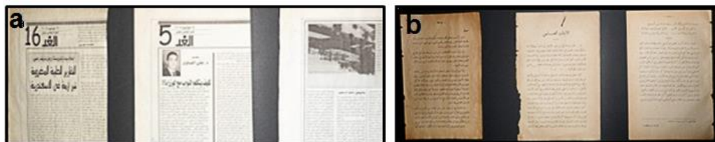
Fig. 3. (A) Acid Newspaper samples (B) Acid Book paper samples, after deacidification Using MMC, Illustrative for color changes to yellowness after artificial ageing
