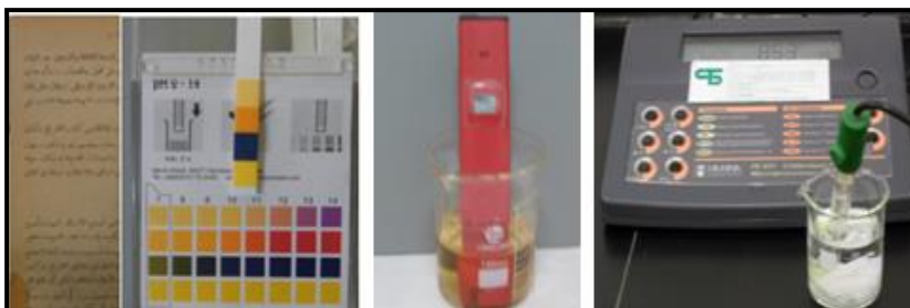
Fig. 4. Measuring of treated samples using the cold water extraction and strips
