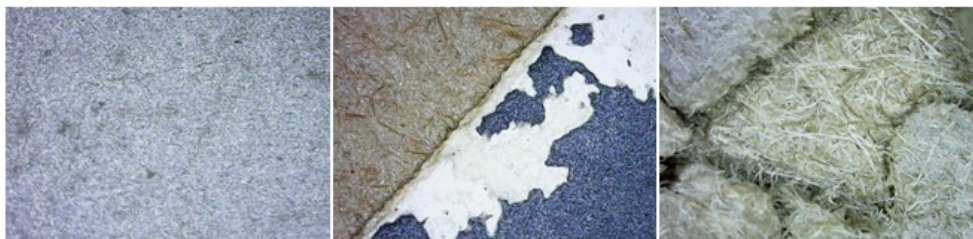
Fig. 9. The silver mirrored surface (left). The baryta coating which is responsible for the absence of the primary support fibers (center). The brittle fibers of the secondary support (right).
