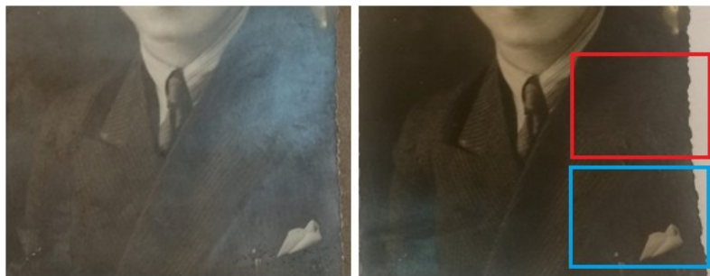
Fig. 3. Photographic sample 1 before treatment (left) and after treatment with pure ethyl alcohol (red square) and after treatment with a solution of 80:20% of ethyl alcohol and distilled water (blue square)
