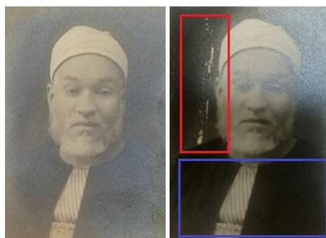
Fig. 5. Photographic sample 3 before coating (left) and after coating with a 2% solution of gelatin in distilled water (right). Generally, good results were obtained (blue square); however, loss in the gelatin binder has occurred in some areas as a result of the treatment (red square)
