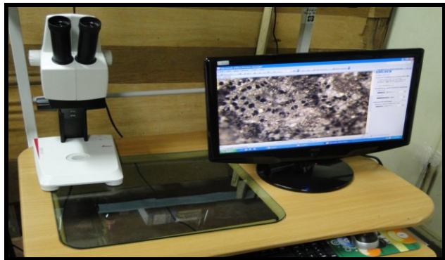
Fig. 4. Leica digital stereoscope used to review and come up with a final identification of wood items examined from all the shrines/landmarks visited
