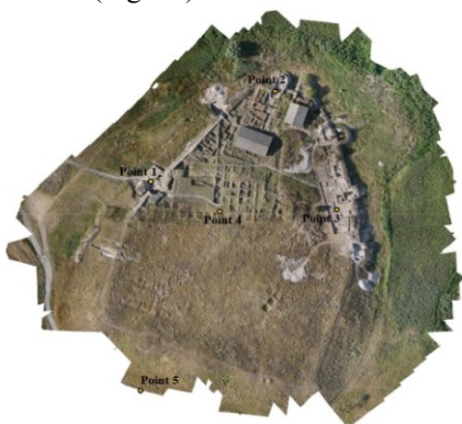
Fig. 12. Locations of the 5 Ground Control Points (GCP)
