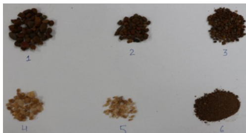
Fig.4. Photograph showing the aggregates of Sindhudurg lime plaster
