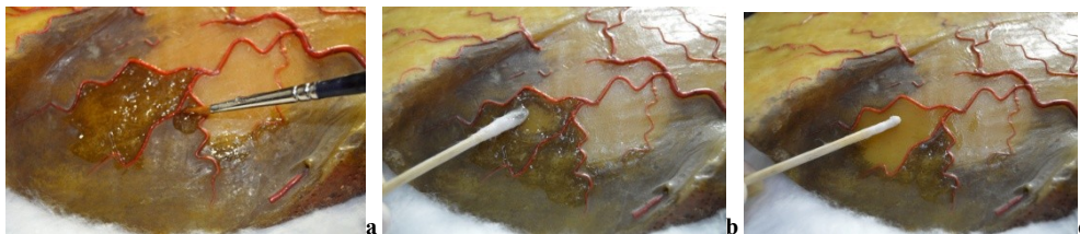
Fig. 6. a. Application of Pemulen® TR2 gel with a brush; b. Process of removing contaminant particles and removal of the gel; c. Final rinse of treated surface
