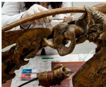
Fig. 3. Gathering data from the model Horse head (MV670): measuring pH and electrical conductivity
