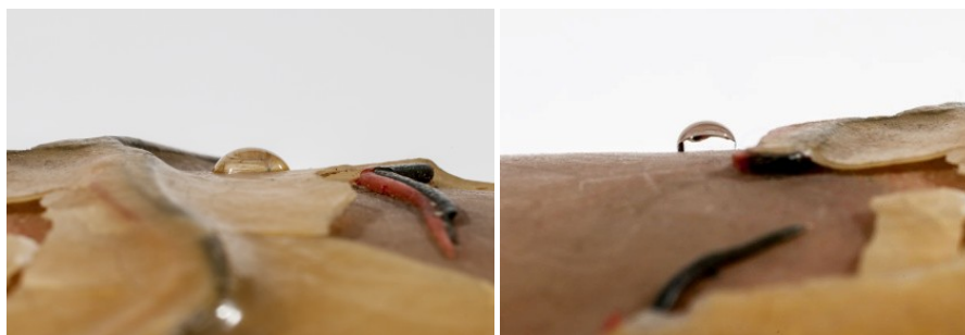
Fig. 2. Testing of contact angle of a drop of water deposited on the wax surface of an anatomical model from the collection: a. drop on the film of coating; b. drop placed directly on the wax
