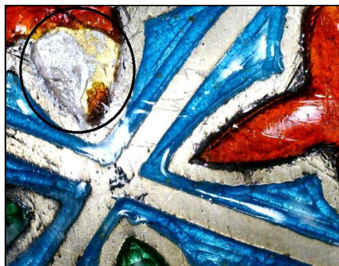
Fig. 12. Digital microscope photomicrograph of the gilding layer beneath the enamel layer.
