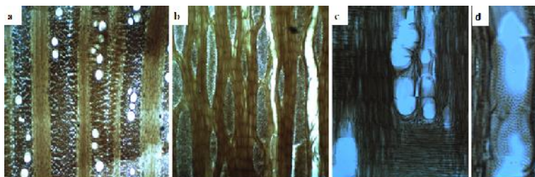
Fig. 3. The anatomical characteristics of Tamarix aphylla by OM in transmitted light: a. Transverse section (TS); b. Tangential section(TLS); c. Radial section (RLS); d. detail of Radial section (RLS) showing simple perforation plates and inter vessel pits alternate
