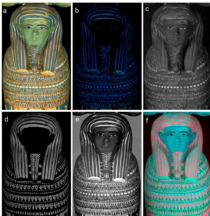
Fig. 4. Technical images of the painted layers made by different spectral ranges using modified Nikon digital camera: a- visible (VIS); b- UV-induced luminescence (UVL); c- UV Reflected (UVR); d- Visible- induced luminescence (VIL); e- Infrared (IR); f- Infrared false color (IRFC).
