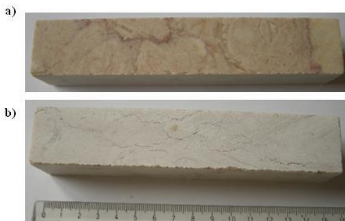
Fig. 1. Lioz limestone with different surface finishes: (a) Polished and (b) Saw cut.
