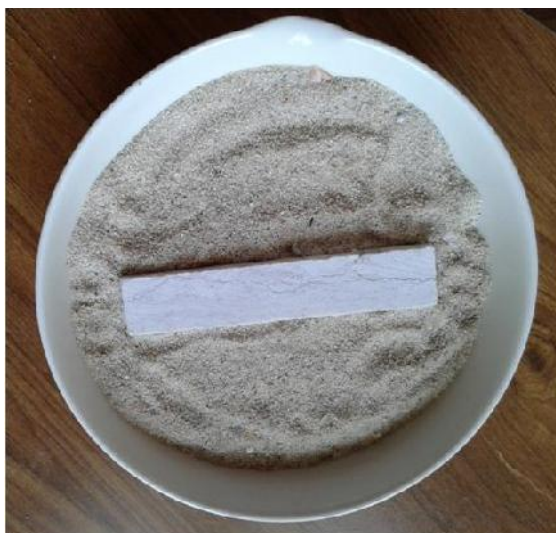
Fig. 2. Sample encased in fine sand.
