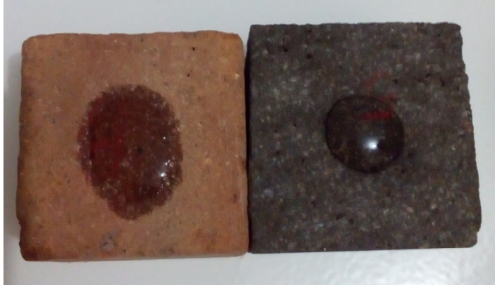
Fig. 9. Comparison cuticle isolation on andesite and brick
