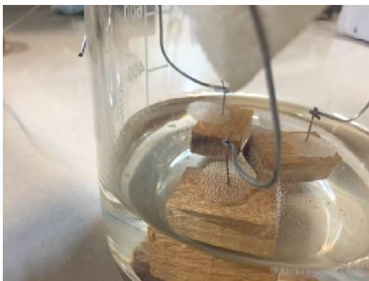
Fig. 1. Immersion of wood samples in the consolidate solution
