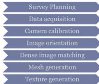
Fig. 2. Workflow for the construction of a 3D model
