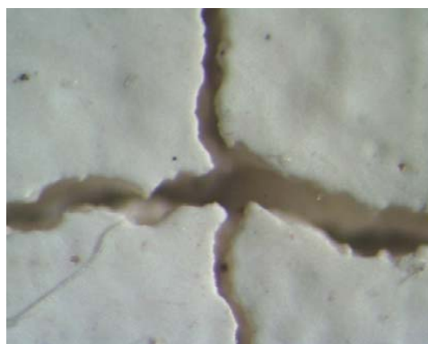
Fig. 4. Microscopic photograph of sample C 4 (aged and consolidated with sturgeon glue, on canvas) after the Thermo Lignum® Warmair treatment (magnification approx. 55 times)
