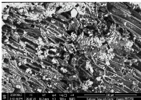
**Fig. 1.** SEM image of longitudinal section of sample no. 1 shows loss in the middle lamella region which causes separations between cells. Loss and erosion in parts of the cell walls are evident.
