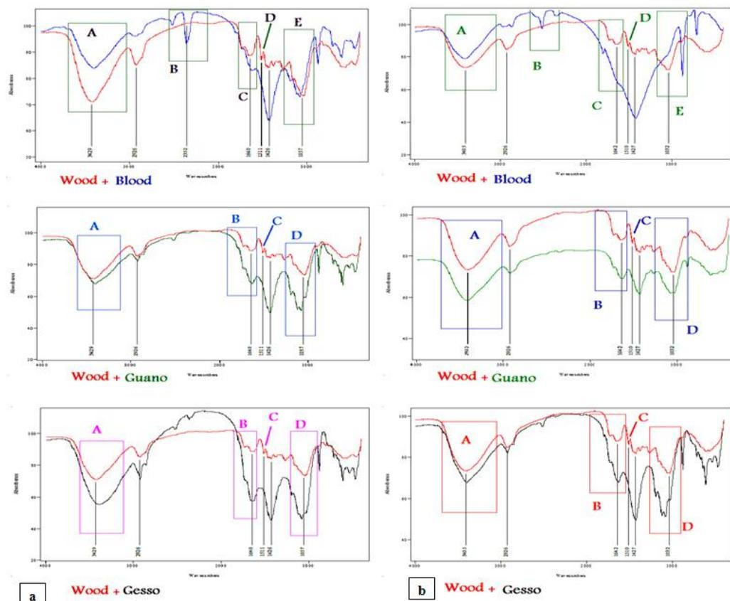
**Fig. 6.** FTIR spectra of wood samples: **a** - from Mohamed Ali's palace showing the alkaline effect of gesso layer and bats' guano on lignin bands which decreased in intensity; **b** - from Baron Empain's palace showing the alkaline effect of gesso layer and bats' guano on lignin bands which decreased in intensity.
