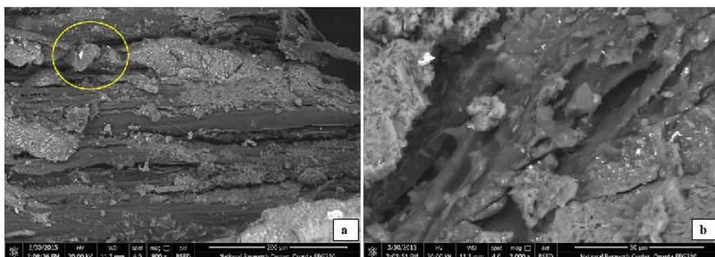
**Fig. 4:** SEM images of longitudinal section of sample no. 4: **a** - shows deterioration of the wood cells due to bats' excretions. Erosion and separations along the cells are obvious. Besides, loss and cracks through the cell walls. Also, this spot was analyzed with EDX; **b** - shows degradation of the cells that lay directly beneath bats' excretions.
