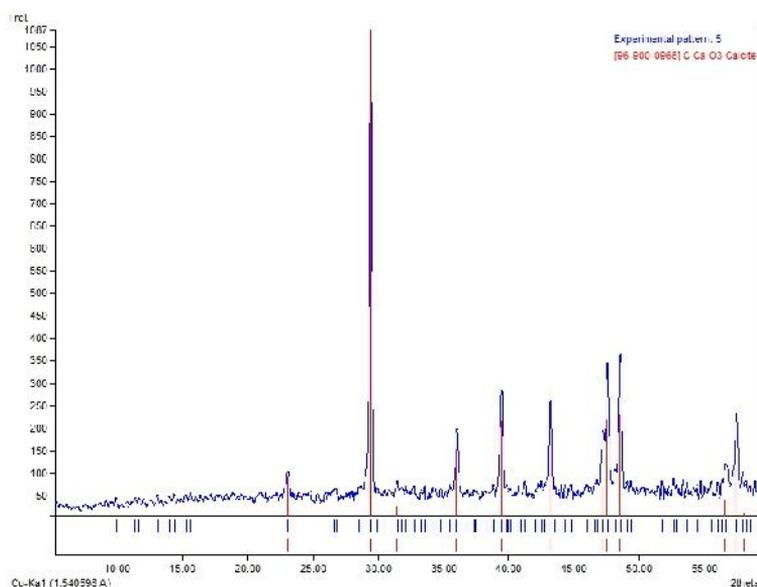
**Fig. 5.** XRD patterns of the studied samples illustrate that calcite is the main component of gesso layer covering their surfaces.
