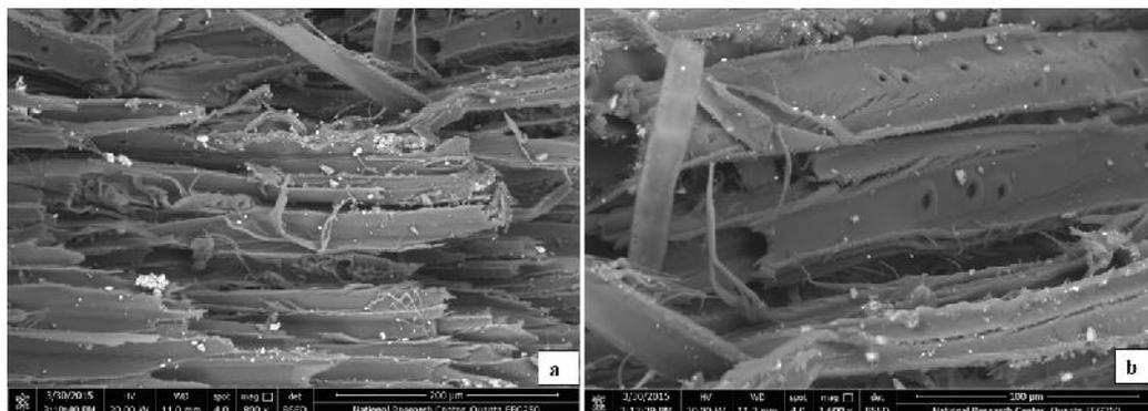
**Fig. 3:** SEM images of longitudinal section of sample no. 3; **a** - shows the wood surface beneath the gesso layer that suffer of loss in the middle lamella region which causes separations between cells. Also, erosion of the cells is evident and caused breakdown in the wood anatomical structure; **b** - showing weakening and disintegration of the wood cells and a series of separations along the cells. Besides, serious cracks, fissures and fractures through the cell walls
