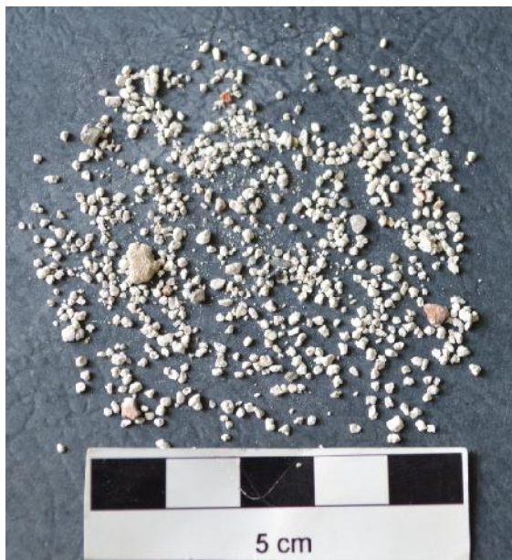
Fig. 8. Showing the types aggregates mixed with the lime mortar of Ballaeshwar temple
