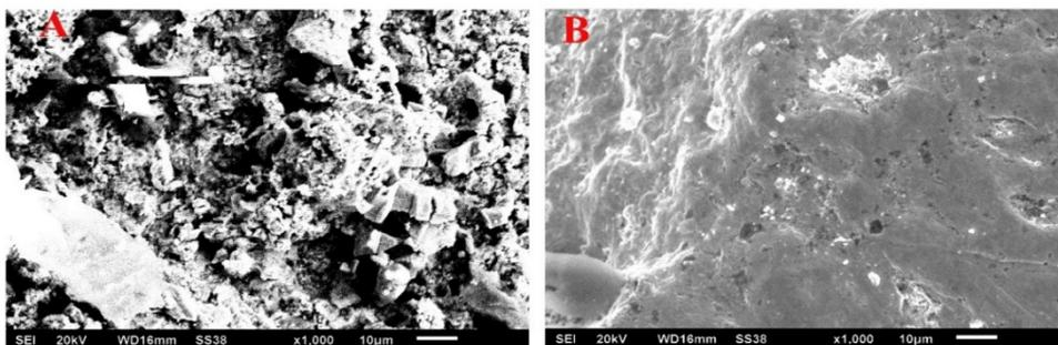
Fig. 10. SEM images of the coin B before and after the laser cleaning:
