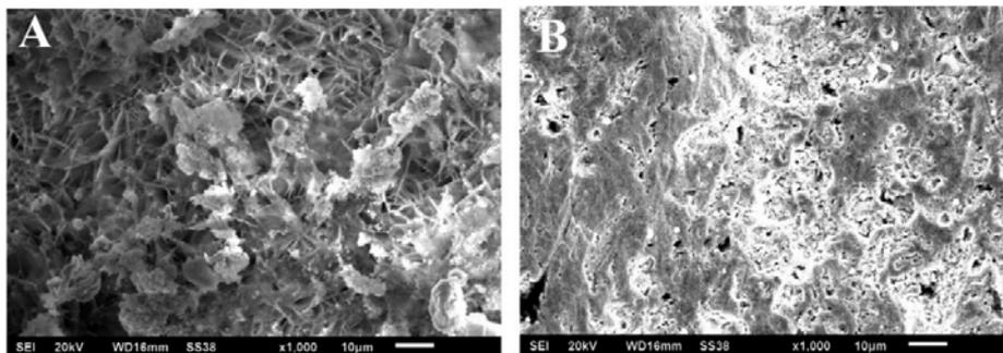
**Fig. 6.** SEM images of the coin A before and after the laser cleaning:
