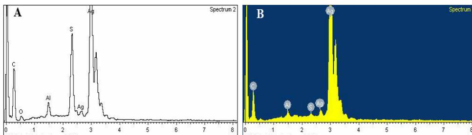
**Fig. 11.** EDX spectrum of the chemical composition (wt. %) of coin B before and after the laser cleaning: A - before the laser cleaning; B - after the laser cleaning
