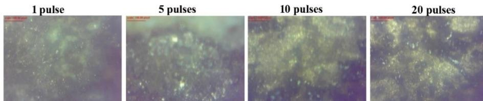
Fig. 4. The effect of cleaning conditions (using defocusing 16cm lens) at a focal length = 10cm) on the surface of Coin A
