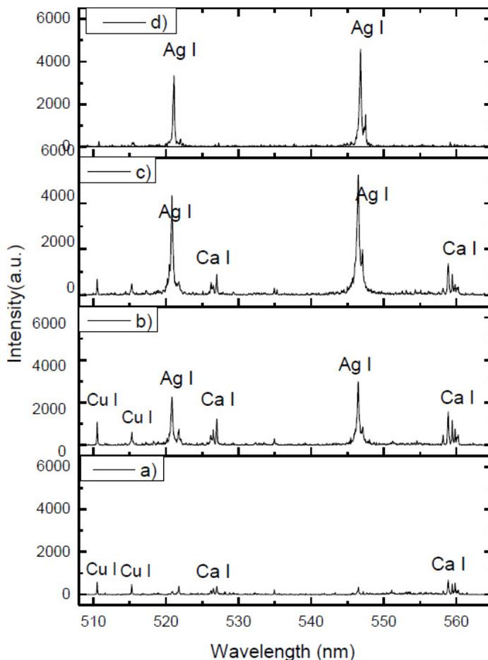
**Fig. 5.** Evolution of LIBS spectra with the number of pulses of coin A by depth profiling on crust for different spectral lines compared with the: a) 1<sup>st</sup> shot; b) 3<sup>rd</sup> shot; c) 4<sup>th</sup> shot; d) cleaned surface
