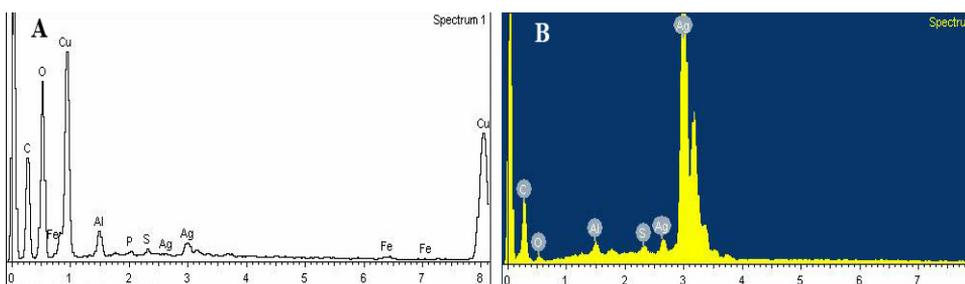
**Fig. 7.** EDX analysis of the chemical composition (wt. %) of coin A before and after the laser cleaning:
