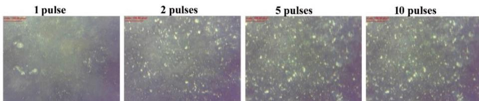
**Fig. 8.** The effect of cleaning conditions (using defocusing 16-cm lens) at a focal length = 10cm) on the surface of coin B
