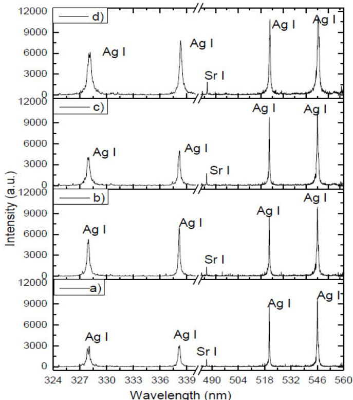
**Fig. 9.** Evolution of LIBS spectra with the number of pulses of sample 14 by depth profiling on crust for different spectral lines compared with the: a) 1<sup>st</sup> shot; b) 2<sup>nd</sup> shot; c) 3<sup>rd</sup> shot; d) cleaned surface
