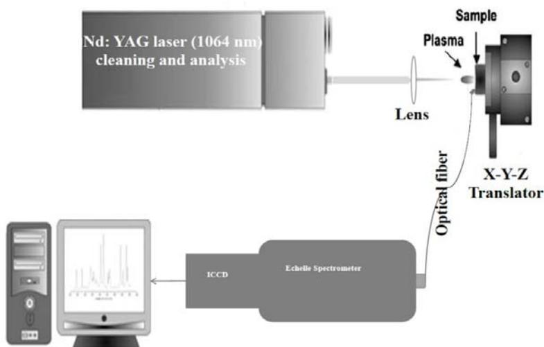
**Fig. 2.** The experimental set-up used in cleaning of coin samples
