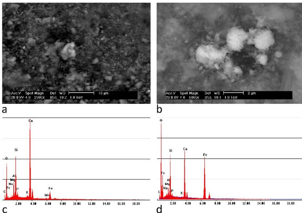
**Fig. 8.** SEM image and EDX spectrum of sample A5: a - area of the surface of red plaster, b - bright particles on the surface of the red plaster, c - EDX spectrum of an area on the surface of the red plaster and d - EDX spectrum of bright particles on the surface of the red plaster
