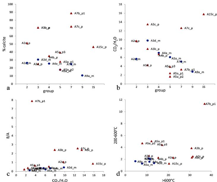
**Fig. 6.** a - % calcite relative to the different groups, b - hydraulicity coefficient relative to the different groups, c - B/A ratio vs. hydraulicity index, relative to the different groups, d - Loss of weight between 200-600°C vs. above 600°C, relative to the different groups. In all the four graphs, circles correspond to mortars and triangles to plasters
