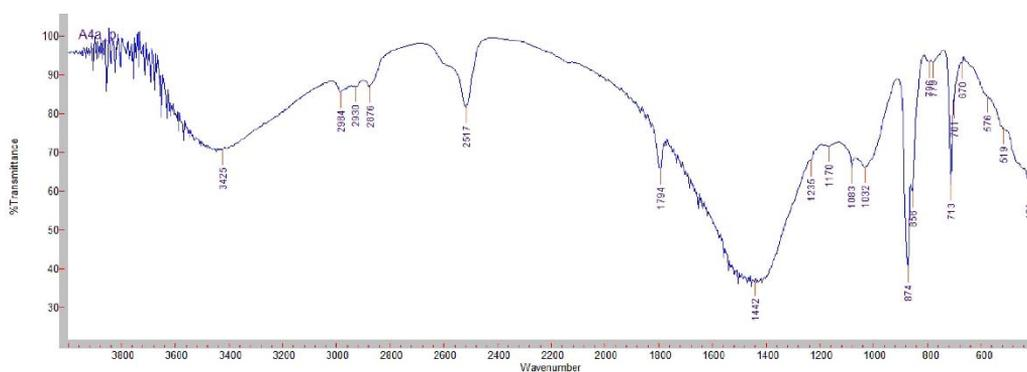
**Fig. 5.** FTIR transmission spectrum of sample A4a\_p in KBr. Peaks of calcite (2517, 1794, 1442, 874, 713 $\text{cm}^{-1}$ ), aragonite (856 $\text{cm}^{-1}$ ), quartz (1083, 796, 779 $\text{cm}^{-1}$ ), silicates (1032, 576, 519, 421 $\text{cm}^{-1}$ ), organic substances (2984, 2930, 2876, 1235 $\text{cm}^{-1}$ ) are noticeable
