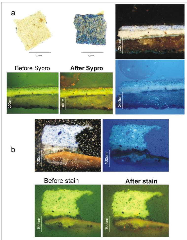
**Fig. 3.** Cross-sections of the samples from the main altarpiece in the Cathedral in Funchal (PT-AM-SFU): a) sample 11 – observed under Vis and UV light, before and after the application of the fluorescent stain Sypro Ruby; b) sample 12 – observed under Vis and UV light, and before and after the application of the fluorescent stain Sypro Ruby.
