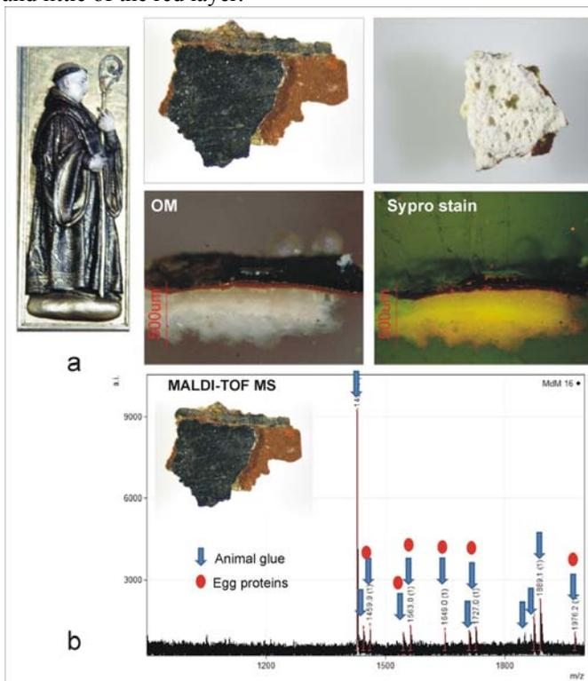
**Fig. 1.** Sample PT-AM-MD-16: a) localisation of sampling, photos of fragment from upper and bottom side and photos of cross-section before and after the application of the fluorescent stain Sypro Ruby; b) MALDI-TOF mass spectrum of the fragment with labelled peaks/peptides coming from animal glue and egg proteins.
