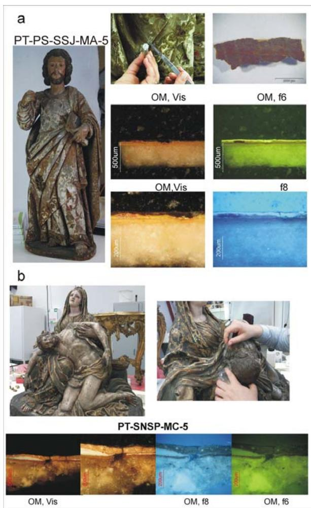
**Fig. 4.** Cross-sections from the two samples taken from two sculptures: a) PT-PS-SSJ-MA-5 – localisation of sampling, photos of fragment from upper side and photos of cross-section in Vis and UV light (f8) and under green filter (f6); b) PT-SNSP-MC-5 – localisation of sampling, photos of cross-section in Vis and UV light (f8), and under green filter (f6).
