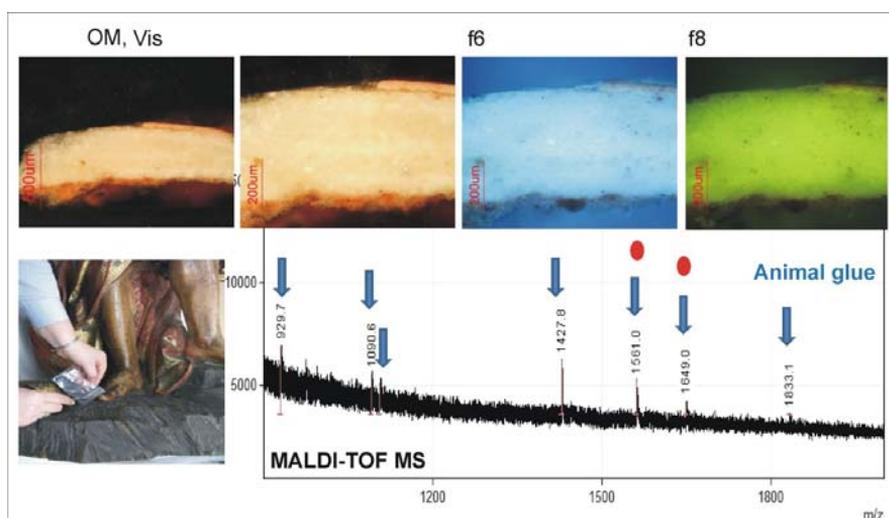
**Fig. 5.** Detection of animal glue using MALDI-TOF MS on sample PT-SNSP-MC-5 from St. John sculpture by Machado de Castro: localisation of sampling, photos of cross-section under Vis and UV light (f8), and under green emission fluorescence (f6).
