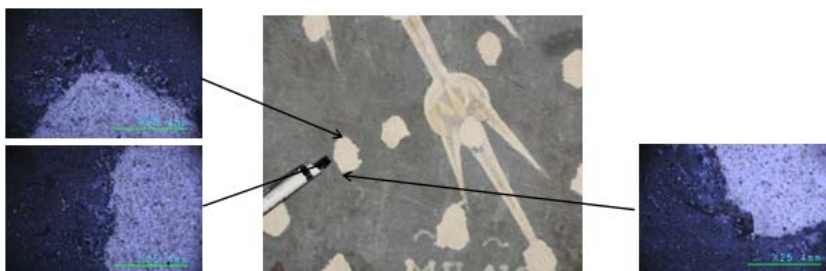
Fig. 2. Microscopic images (25X) for one of the filled gaps
