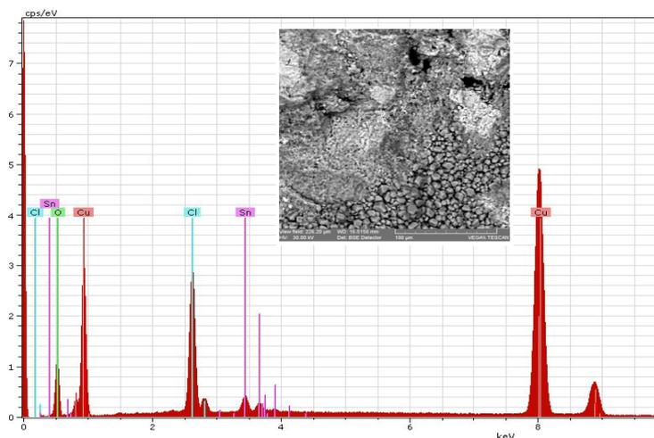
Fig. 6. The SEM microphotography and the EDX spectrum for S2
