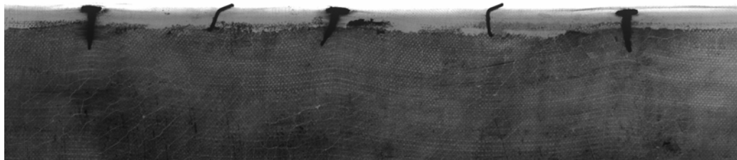
Fig. 10. Detail of the radiograph showing the canvas distortion and the old nails (along with recent bent nails). For better visibility, the radiograph negative is presented.
