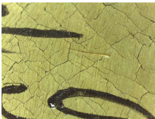
Fig. 5. Marks and hair left by the brush on the varnish surface in the area of the paper with the inscription. The inscription was applied over these marks.
