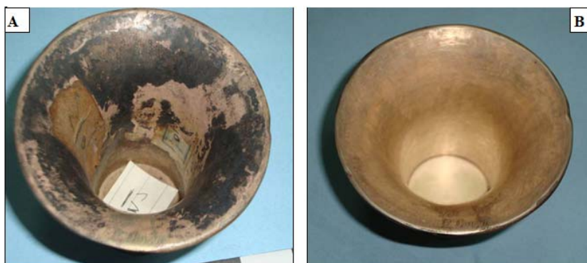
Fig. 12. Interior surface of silver object no.28: a - before treatment; b - after treatment
