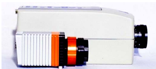
Fig. 4. Xenics Bobcat 640 is about 4 times smaller than the Indigo System Merlin camera
