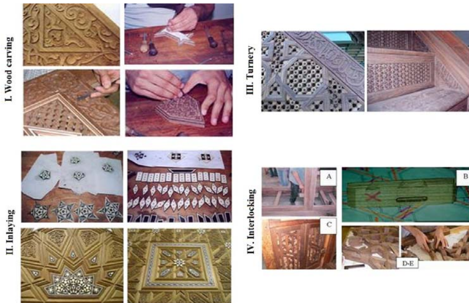
Fig. 6. The implemented traditional craft techniques: Wood carving, Inlaying, Turnery, Interlocking (A – Cotters, B – Click & tongue, C – cotters connecting side door with the minbar body, D, E – interlocking of wooden pieces of chords), source: Applied Balqa University.
