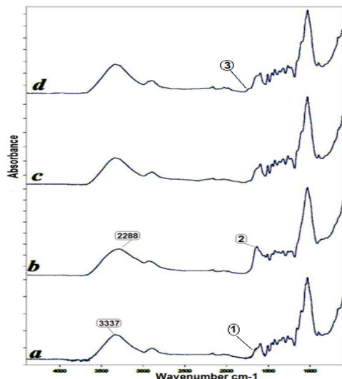
**Fig. 6.** FTIR spectrum of the reference sample (a), wood inoculated with *Botryodiplodia theobromae* (b), wood inoculated with *Trichoderma longibrachiatum* (c), and wood inoculated with *Aspergillus terreus* (d), indicating the following bands:
