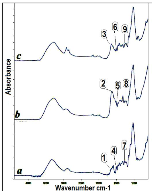
**Fig. 7.** FTIR spectrum of the reference sample (a), wood inoculated with *Aspergillus candidus* (b), wood inoculated with *Aspergillus ustus* (c), indicating the following bands; 1, 2 and 3 - conjugated C=O bands at 1640 cm<sup>-1</sup>, 4, 5 and 6 - aromatic >C=C< stretching bands at 1509cm<sup>-1</sup>, 7, 8 and 9 - C-O-R stretching bands at 1263cm<sup>-1</sup>
