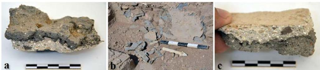
**Fig. 9.** MP.2 sample showing the two layers (the white layer and the grayish layer): a and c - cross section, b - the area where MP.9 sample was taken from.
